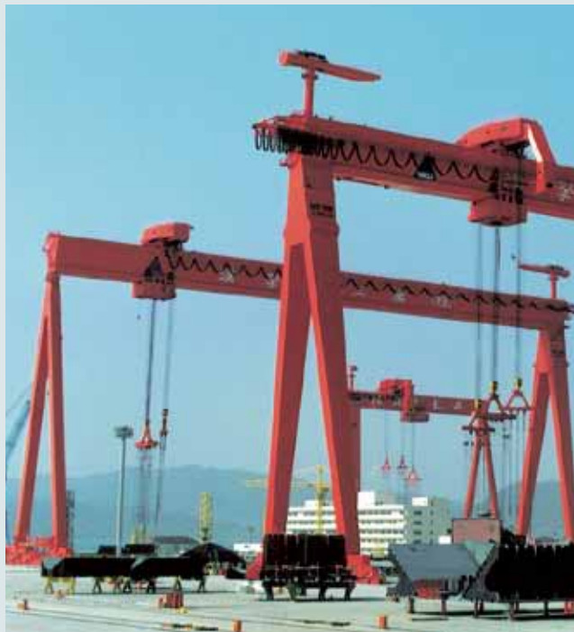
Single girder construction 600 t / 175 m
