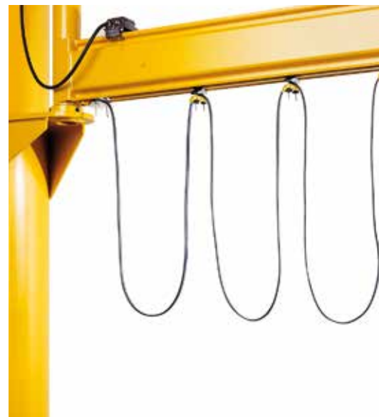
Hoist power feeding, flat cable under the profile
