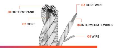
Typically, only 20% of the rope can be inspected visually, while the core remains complete inaccessible for such inspection.
