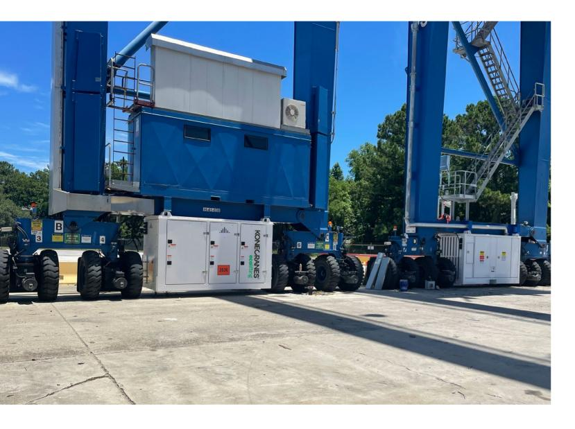
At the Wando Welch Terminal in Charleston, South Carolina Ports (SC Ports) has had 12 of their Konecranes RTGs upgraded with an EPA-approved Konecranes hybrid retrofit. These cranes now have reduced fuel consumption and lower carbon emissions with easier maintenance while retaining the same level of operational performance.
