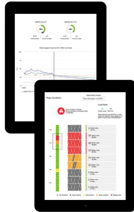
Top: TRUCONNECT Brake Monitoring data on Konecranes Portal. Bottom: TRUCONNECT Wire Rope Monitoring data on Konecranes Portal.
