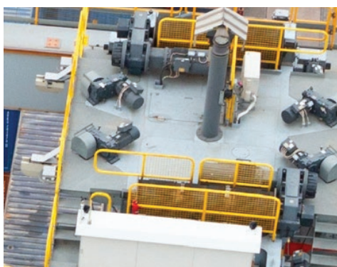
Service hoist for typical 16W RTG trolley (one jib)
