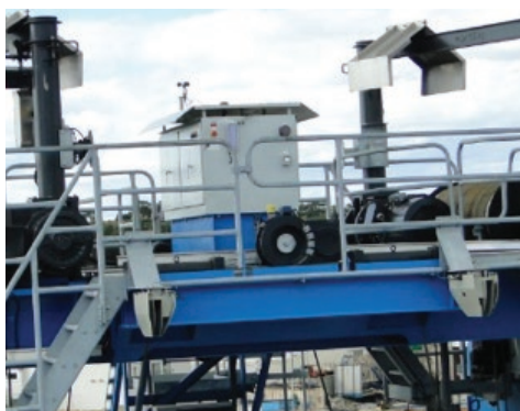
Service hoist for typical 8W RTG trolley (two jibs)
