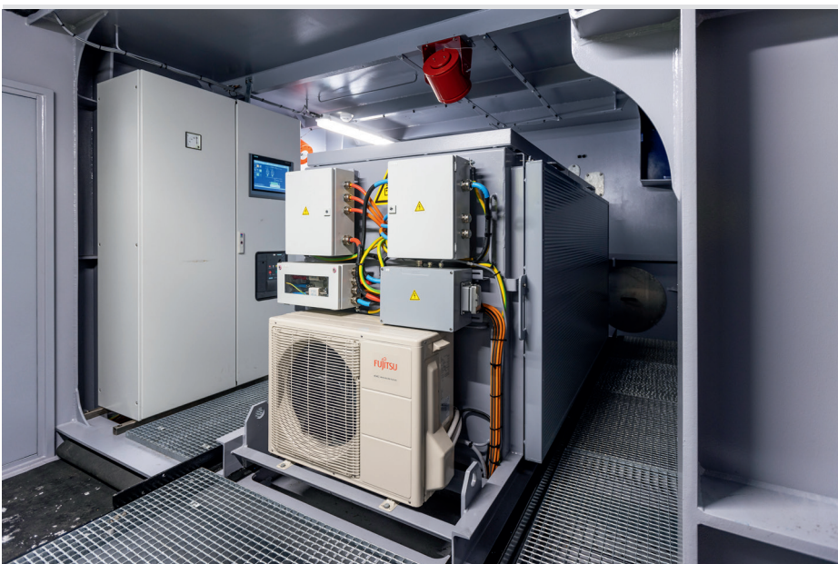
The Model 6 mobile harbor crane is equipped with a 250 kWh battery pack to move and operate the crane unplugged
