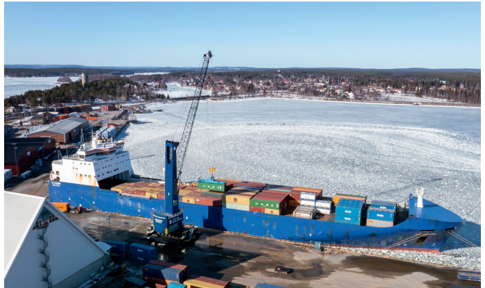
The all-electric Konecranes Gottwald Mobile Harbor Crane with battery drive handles containers in the Port of Skellefteå to support the new battery plant
