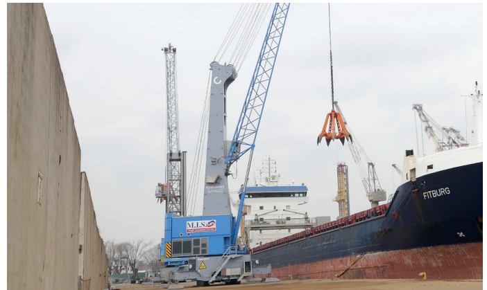
Backbone and backup: the HMK 330 EG can quickly come to the aid of the G HMK 6507 B as soon as the situation requires it.
